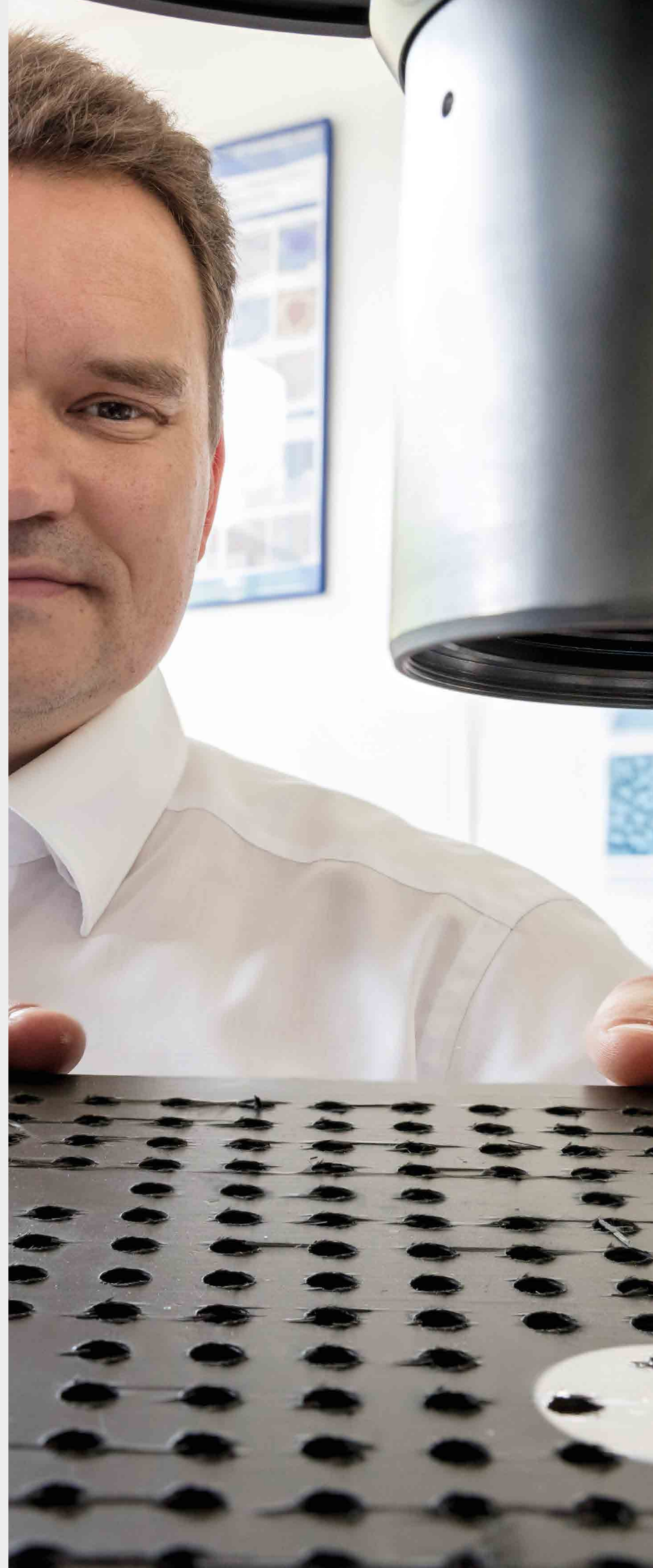
Dieter Meinhard inspects holes drilled in CFRP using drill bits with varying degrees of sharpness.
