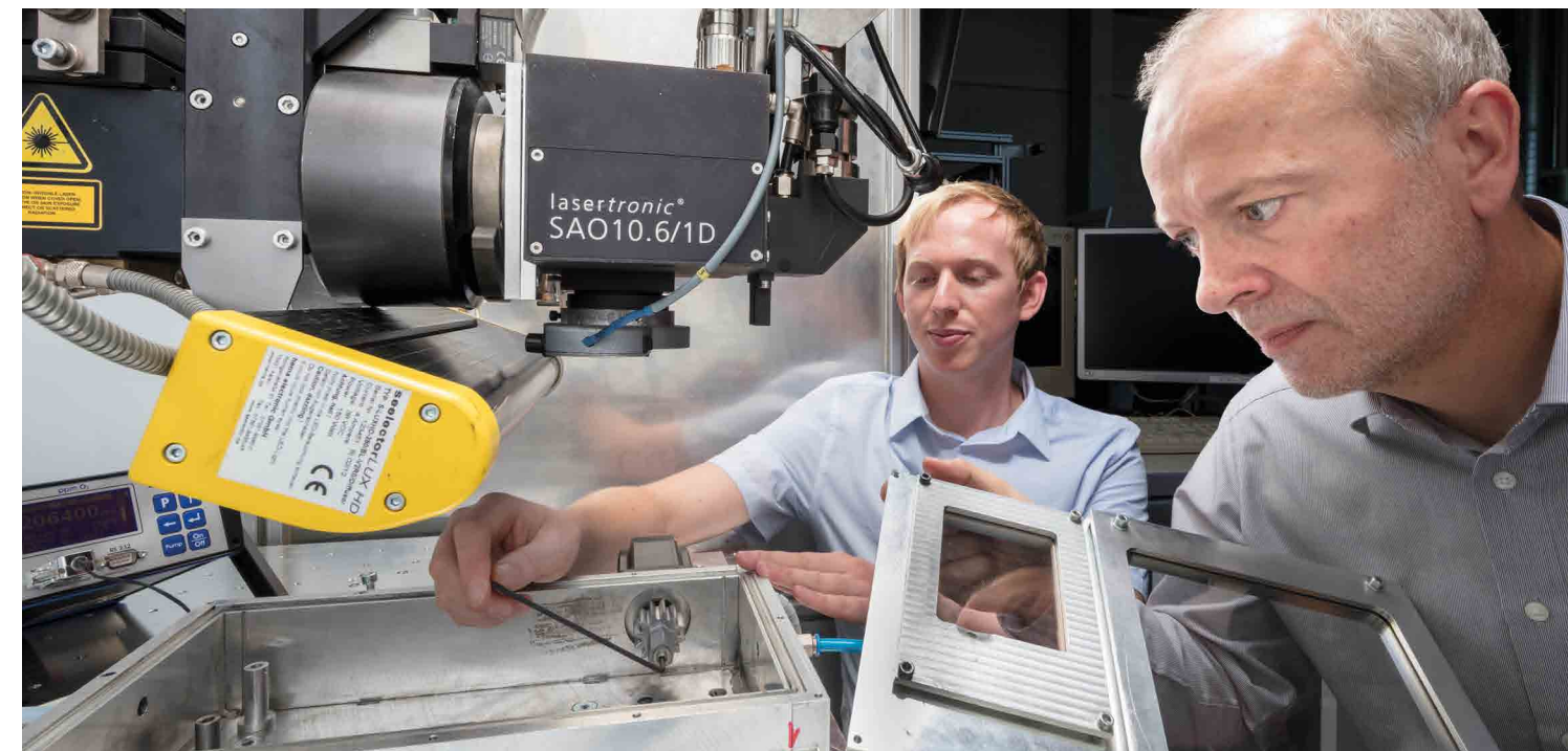
Lasers instead of rags: Harald Riegel (right), head of the Laser Application Center, and doctoral student Simon Ruck clean the surfaces of printed components in the lab using light from a laser.
